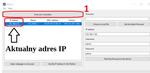
Fig.7 Searching for the current IP address of a device in LKTools program
