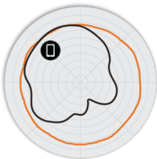
Figure 2. H510 2.4GHz Azimuth Antenna Patterns
