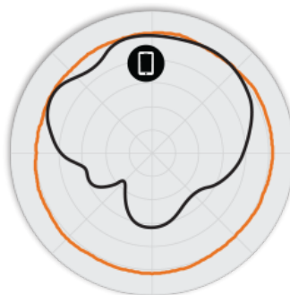
Figure 3. H510 5GHz Azimuth Antenna Patterns
