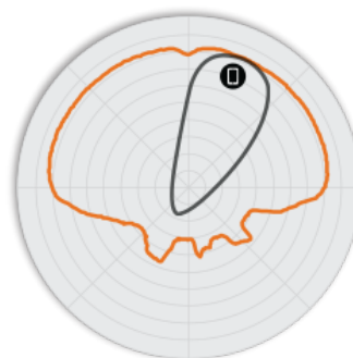
Figure 4. H510 2.4GHz Elevation Antenna Patterns
