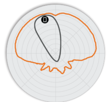
Figure 5. H510 5GHz Elevation Antenna Patterns
