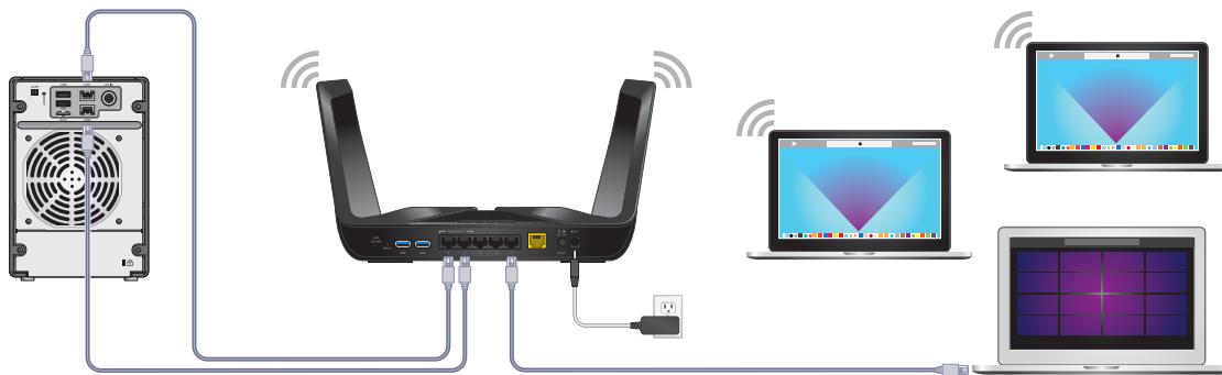
Figure 7. Ethernet port aggregation
