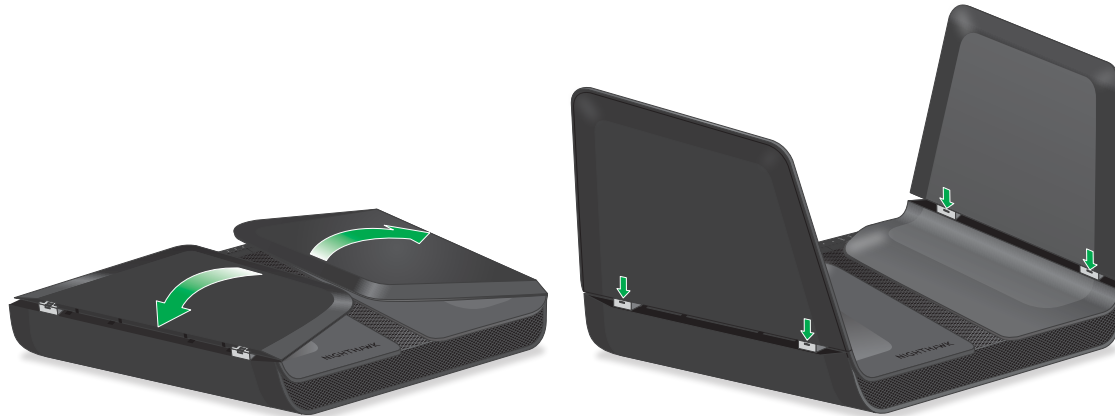
Figure 4. Position the antennas
