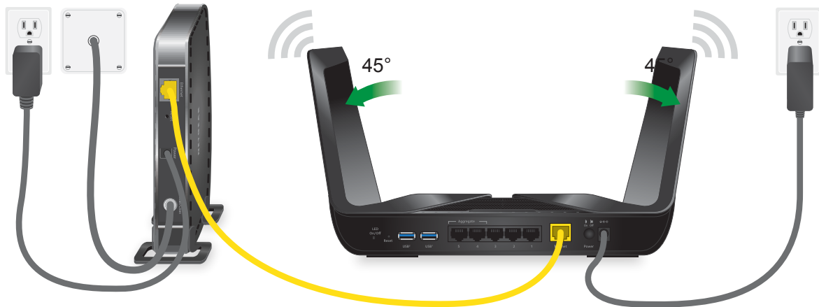
Figure 6. Cable your router
