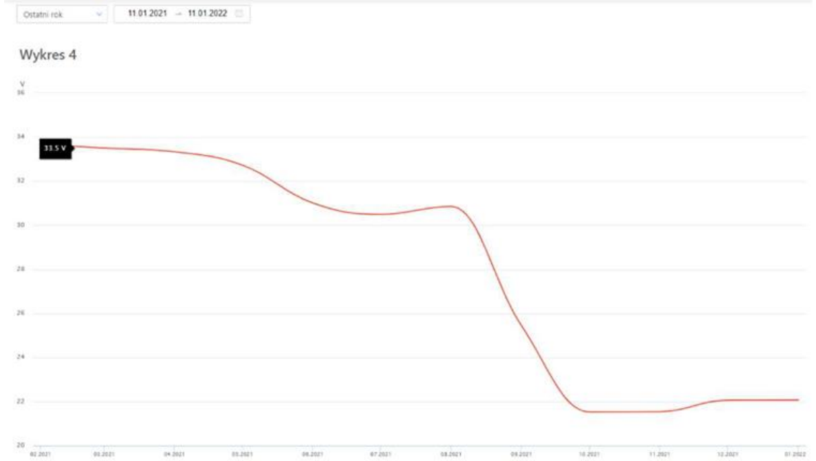
Fig.3 Screenshot from the Solar Edge monitoring application with a visible drop in power
