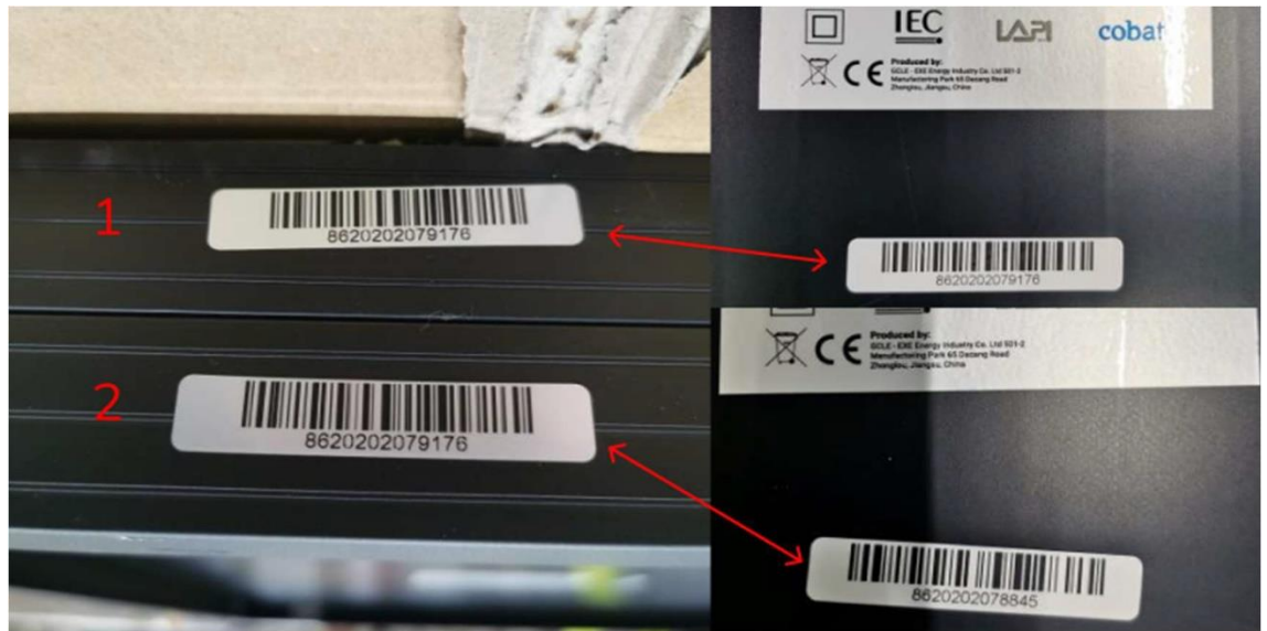
Fig.2 Duplicate and incorrectly attached serial number
