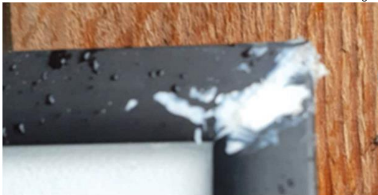
Fig.5 Silicone residues from the production process
