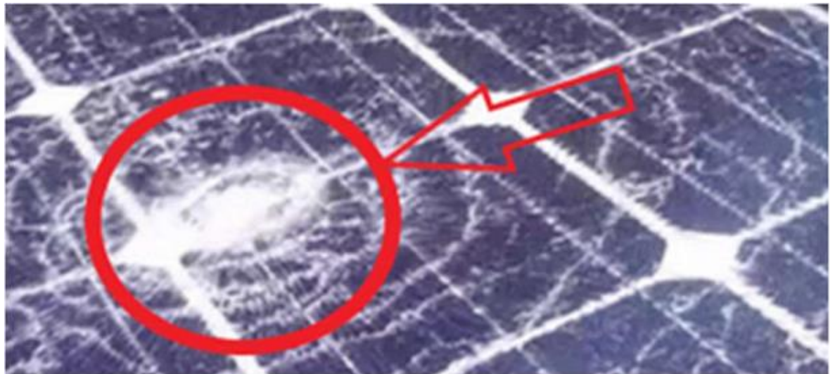
Fig. 2 Fracture caused by an external factor
