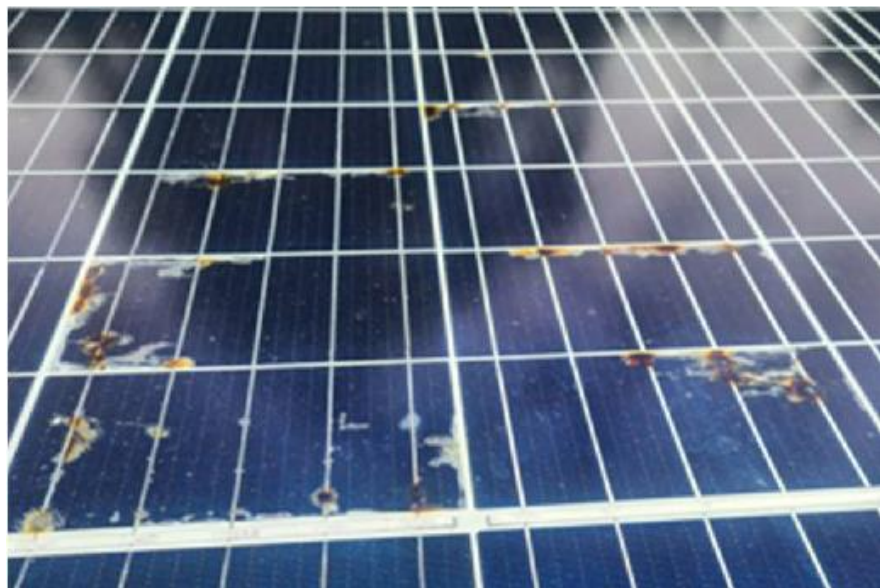
Fig.2 Visible spot burns
