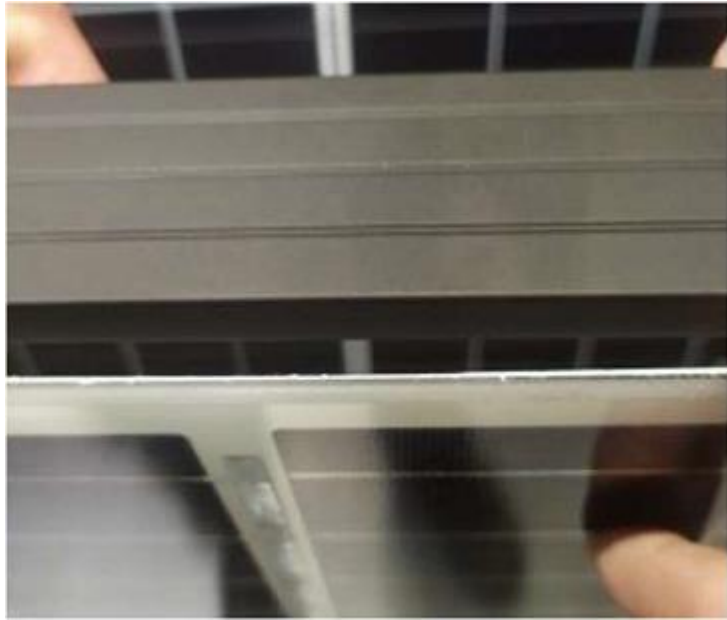
Fig.5 Air bubble under the glass
