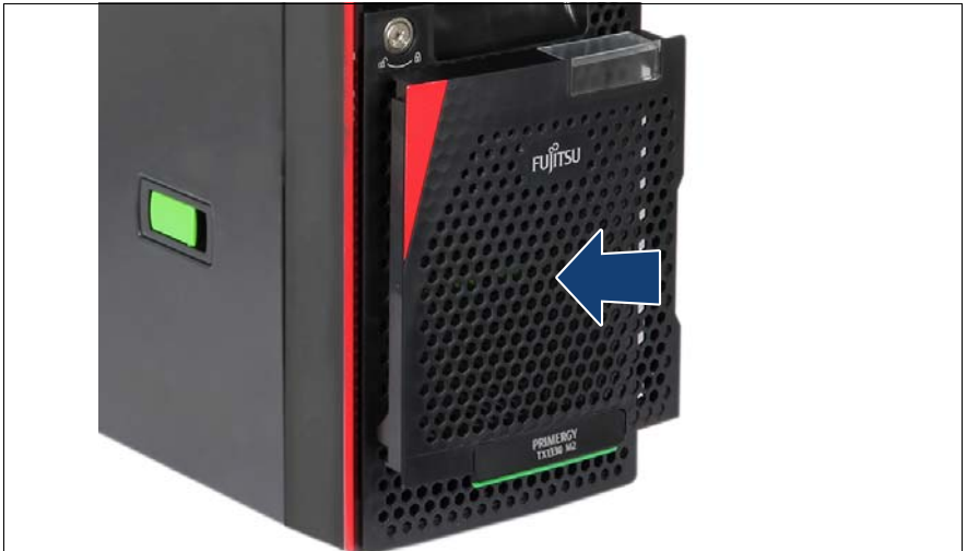
Figure 22: Placing the accessible drive bay cover
