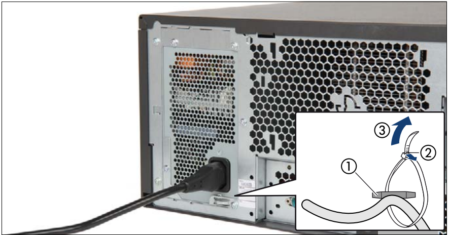
Figure 19: Securing power cord
