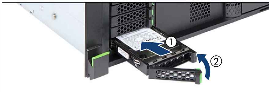
Figure 26: Installing the 2.5-inch HDD/SSD module
