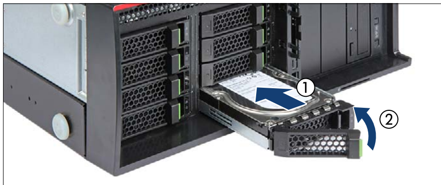
Figure 29: Installing the 3.5-inch HDD module
