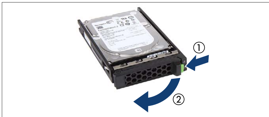
Figure 25: Opening the 2.5-inch HDD/SSD module locking lever
