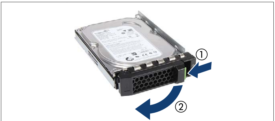
Figure 28: Opening the 3.5-inch HDD module locking lever
