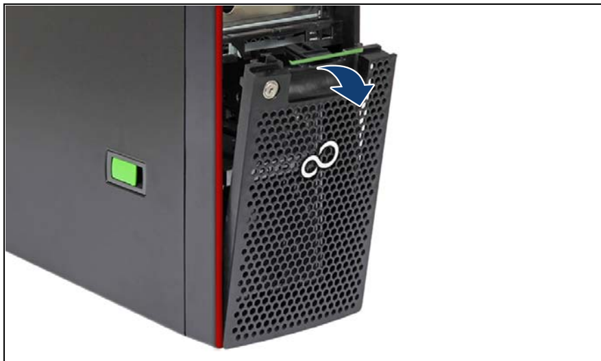
Figure 23: Removing the HDD bay cover
