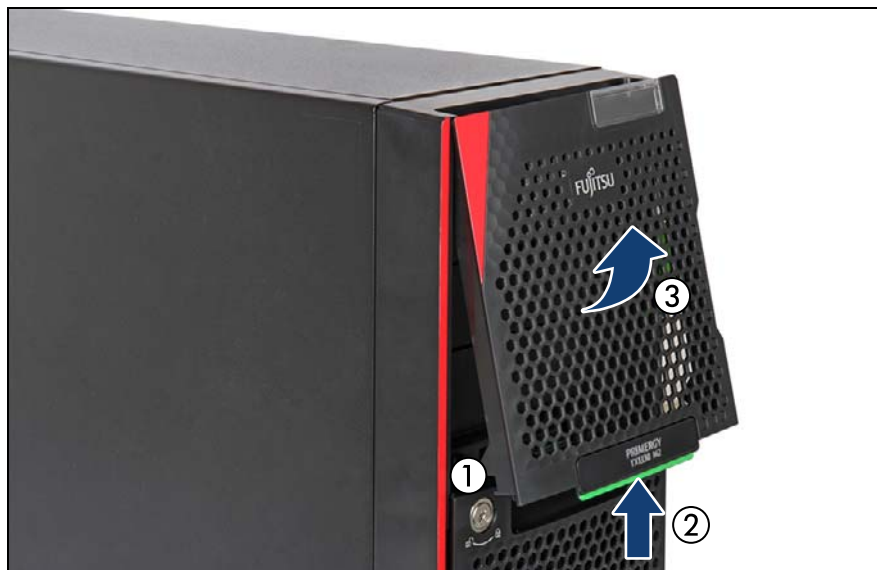
Figure 21: Removing the accessible drive bay cover
