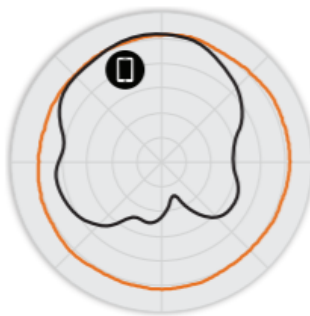
Figure 4. C110 2.4GHz Elevation Antenna Patterns
