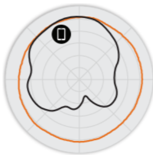
Figure 3. C110 5GHz Azimuth Antenna Patterns
