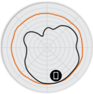
Figure 2. C110 2.4GHz Azimuth Antenna Patterns
